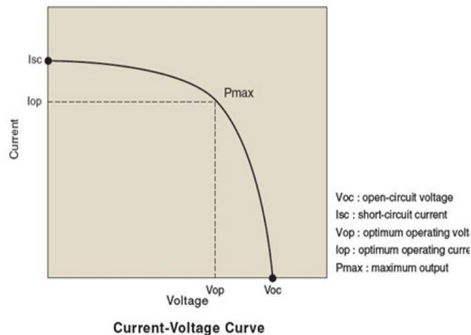
Figure 4. Typical Power Profile of a Photovoltaic Cell
