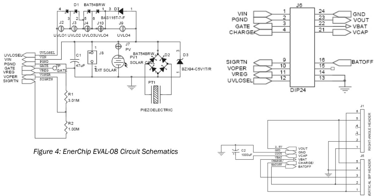
Figure 4: EnerChip EVAL-08 Circuit Schematics
