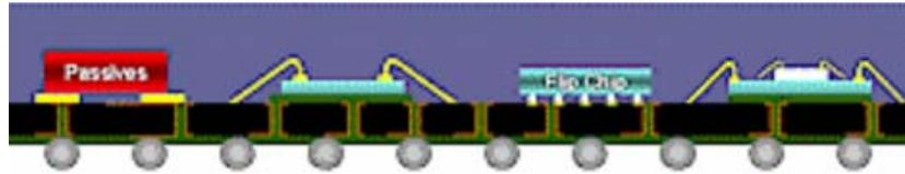
An important attribute of Solid State Energy Storage built on silicon wafer is that they can be solder attached to the circuit board surface using a “flip chip” technique. The flip chip attachment mechanism opens up many new miniature packaging options.
