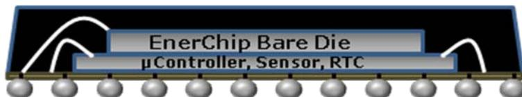
Rechargeable Solid State Energy bare die in System on Chip module:
