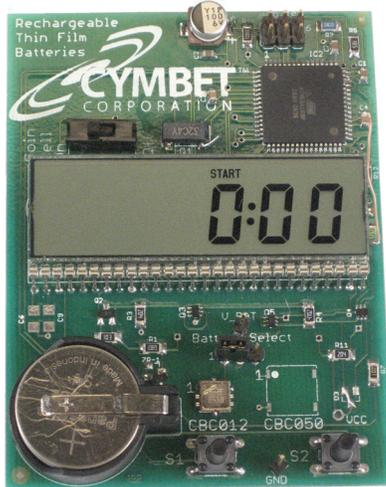
Figure 1. Cymbet Atmel picoPower AVR Demo Board.
