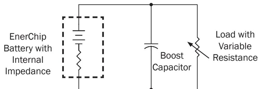
Figure 1. EnerChip with External Capacitor to Supplement Power to the Load.
