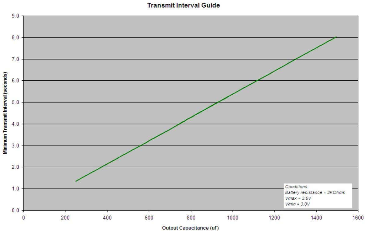
Figure 7. Transmitter Intervals Required for a Given Output Capacitance.
