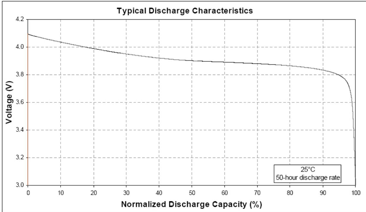
Figure 4. Typical EnerChip Discharge Profile.
