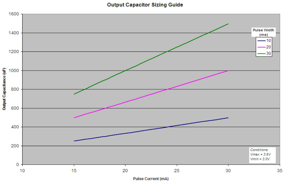
Figure 6. Output Capacitance Required for Typical Transmitter Pulse Currents.
