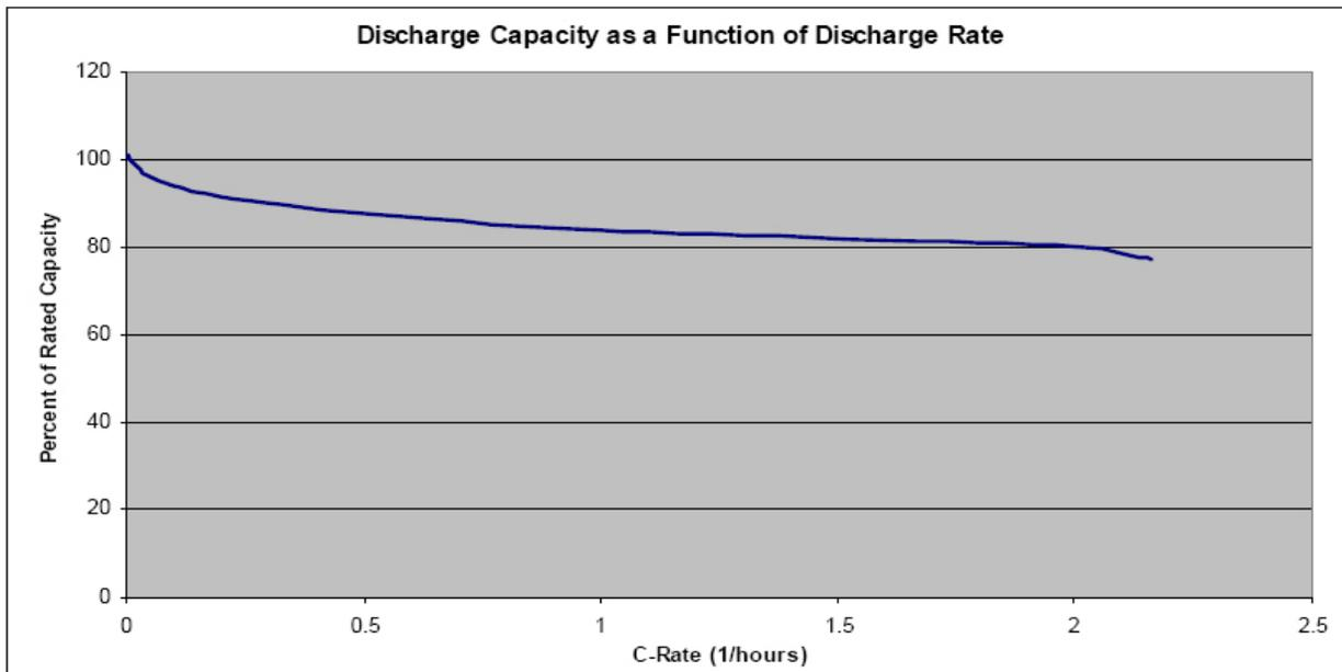
Figure 2. EnerChip Discharge Capacity at Various Discharge Rates.
