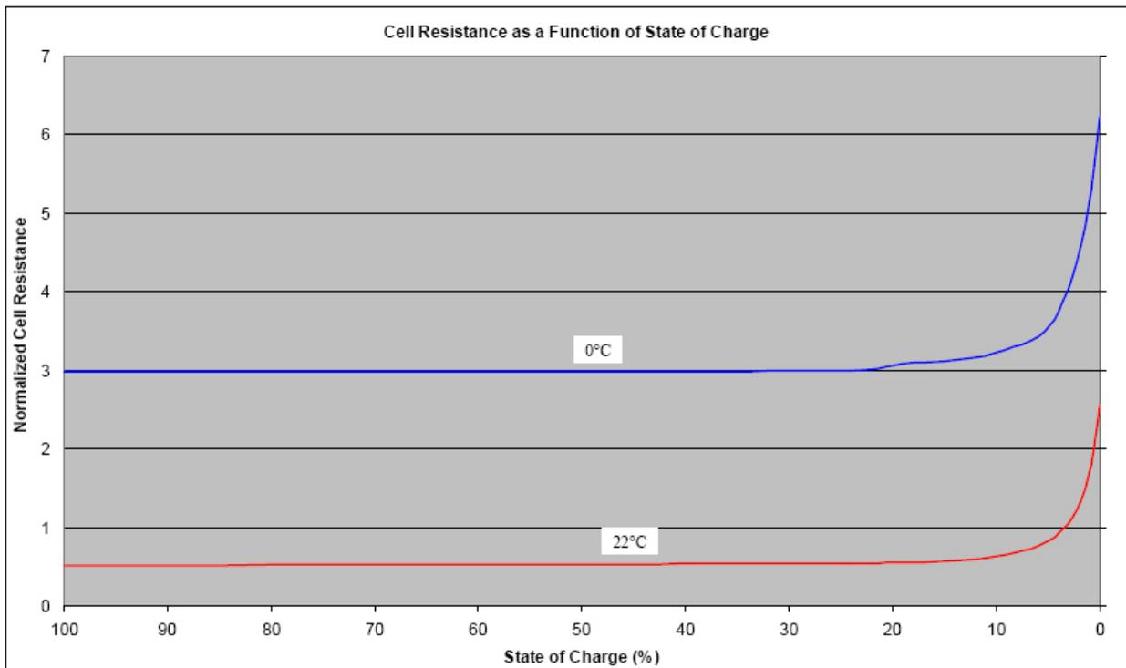
Figure 3. Dependence of Cell Resistance on State-of-Charge.
