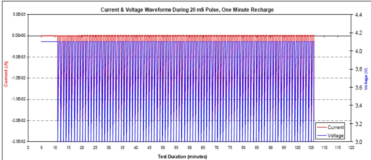
Figure 5. Pulse Discharge Current and Voltage Waveforms. EnerChip CBC050 with 1000 $\mu$ F Capacitor in Parallel.
