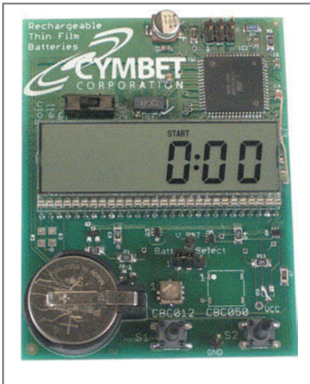
Photo 2 —This design shows how EnerChips and coin cell batteries can work together. [4] The EnerChip keeps the system alive when the coin cell needs to be replaced.
