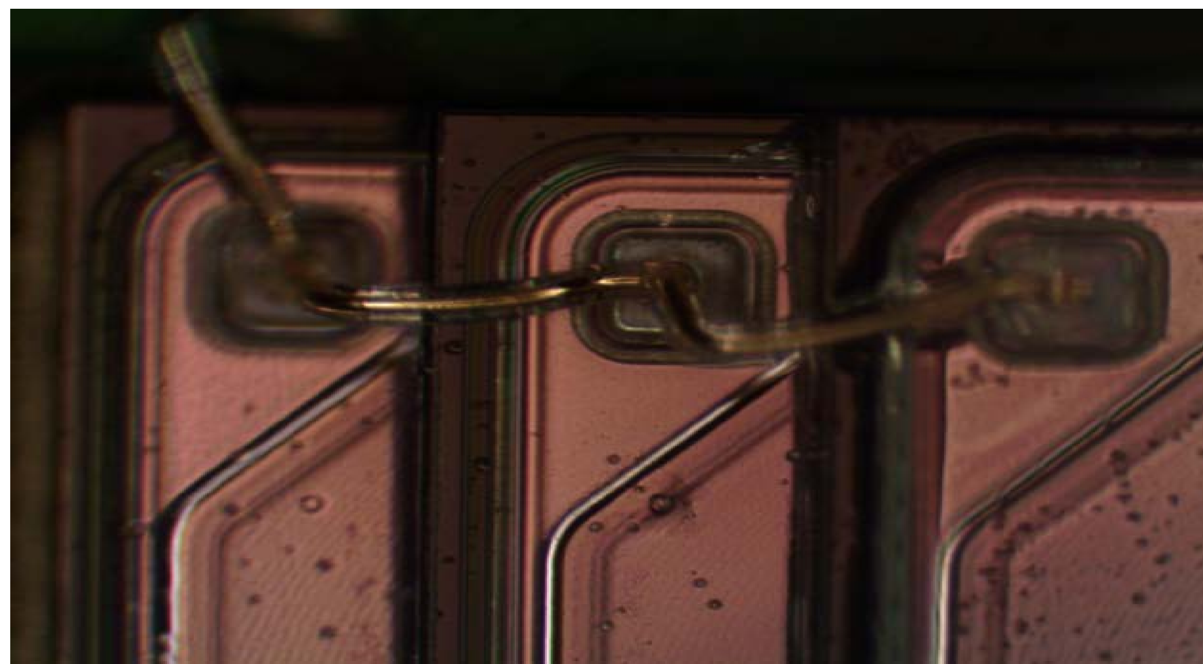
Three Stack Waterfall Wire bond 700 micron height
