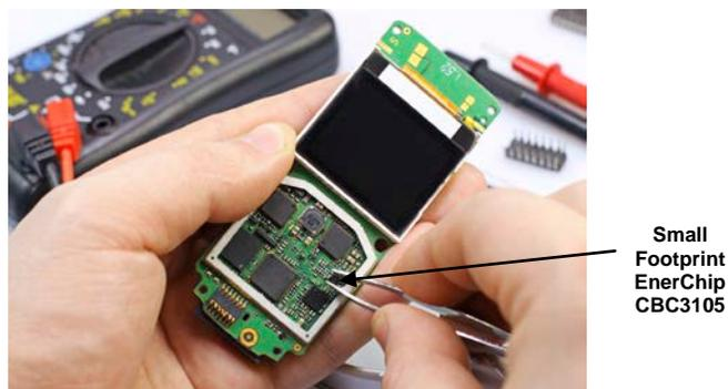
*Figure 3: EnerChip CBC3105 used in a Mobile Phone Secondary Battery Application*
