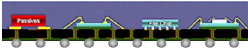
An important attribute of Solid State Energy Storage built on silicon wafer is that they can be solder attached to the circuit board surface using a “flip chip” technique. The flip chip attach mechanism opens up many new miniature packaging options.
