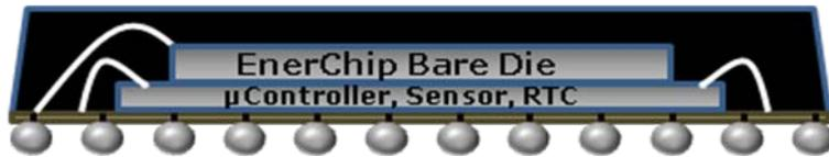
Rechargeable Solid State Energy bare die in System on Chip module:
